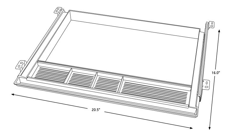
Note: Brackets mount in outboard position under work surface for application widths 29" or greater, and in the inboard position for widths less than 26.7"
