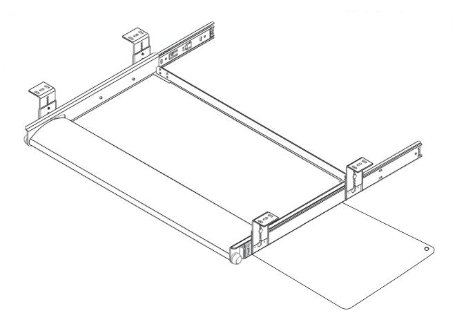
Note: Brackets mount in outboard position under work surface for application widths 24" or greater, and in the inboard position for widths less than 24"
