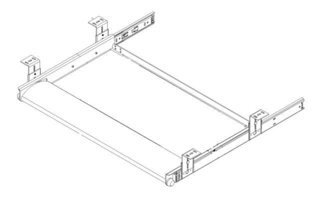
Note: Brackets mount in outboard position under work surface for application widths 24" or greater, and in the inboard position for widths less than 24"
